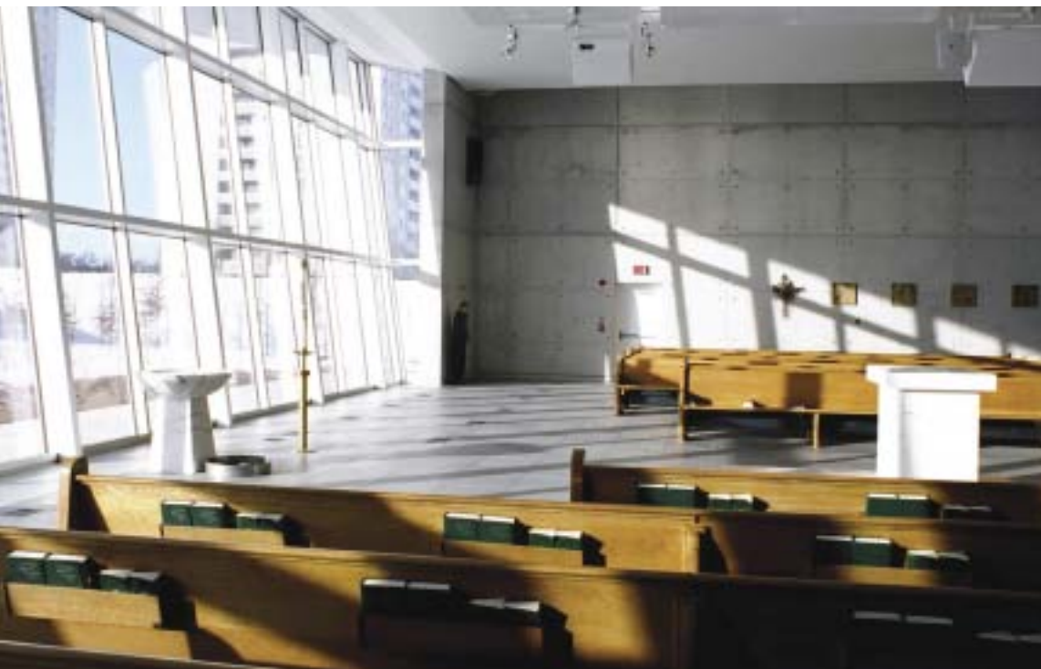
In winter, the south-facing glass wall of St. Gabriel's harvests the sun's heat and light energy.
