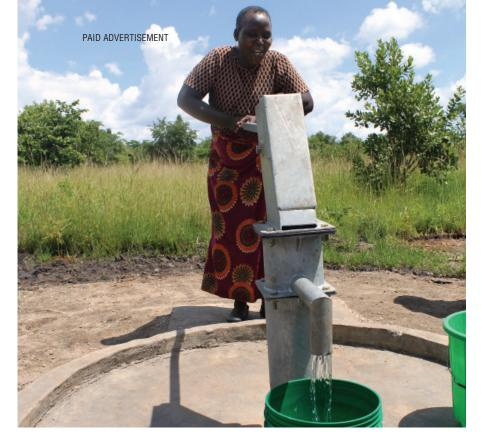
technology or complex processes. The solution typically begins with the installation of a standard well and a simple system to deliver the water to a community distribution point. The hardware works on simple mechanics and is easy to maintain once local families are trained to care for it.
